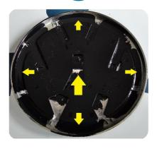
Press the badge firmly onto the face of the Van-Plug and tape down until the adhesive has cured.
