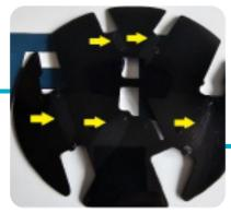
Apply adhesive to the areas that will line up with the backplate first. Carefully line up, press into place and allow to cure. Be careful not to use too much adhesive, as it will seep onto the visible area.
