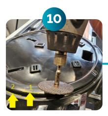
Using a mini disc cutter, remove the first section of the badge retaining plate. Cut to the edge marker '1' first
