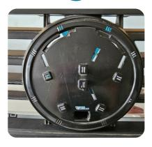
(On the T5.1 they will need to be cut back to 3mm maximum). Use snips or a multi-tool to cut them back.
