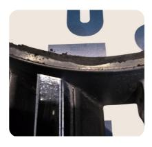
Using a round edge file, smooth out the edges, leaving between 3-6mm of flange.
