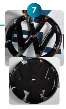
Once cured, apply adhesive to the remaining outer ring on the underside and in the centre as shown.
