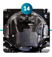
Remove the clamps and 'hook' the top locator into place, then add the three clamps.
