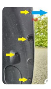
Unscrew the two T25 screws under the wheel arch and the two trim studs. Release the side panels of the bumper from the wings by gently pulling them outwards.
